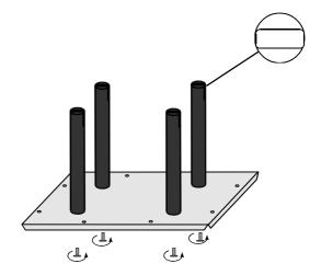
3. Remove the Philips head screws from the handles.
